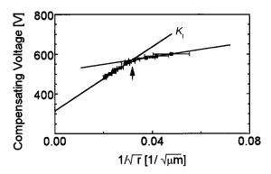
FIG. 5. Electric potential ahead of the crack tip plotted vs  $1/\sqrt{r}$  for a 30-mm-long crack at a crack intensity of  $K_I = 1.6 \text{ MPa} \sqrt{m}$  after 4.4 mm crack advance at crack velocity  $10^{-5} \text{ m/s}$ .
