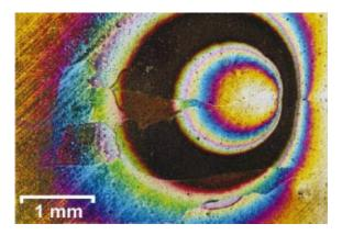
FIG. 3. (Color) Process zone potential field for a fully developed process zone before crack advance in the compensating twisted nematic mode.
