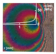
FIG. 2. (Color) Stress-generated electric potential contours prior to development of a plastic zone and crack advance in a poled ferroelectric compact tension specimen displayed by the floating potential mode. The crack tip is located at the origin of the inset. The elastic stress ahead of the crack is delineated ( $K_I$ =0.5 MPa $\sqrt{m}$ ).
