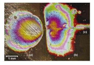
FIG. 4. (Color) (a) Elastic-plastic stress field ahead of the crack tip, (b) modification of the elastic stress field due to the process zone, and (c) the remanent polarization of the process zone outside the elastic stress field of the crack tip in the quantitative compensating twisted nematic mode.
