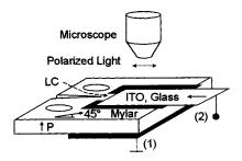
FIG. 1. Liquid-crystal display of the stress field in a ferroelectric compact tension specimen (see Ref. 14): (1) back electrode and (2) transparent electrode at fixed or floating potential. The arrows indicate the liquid-crystal orientation on each surface for the twisted nematic mode.
